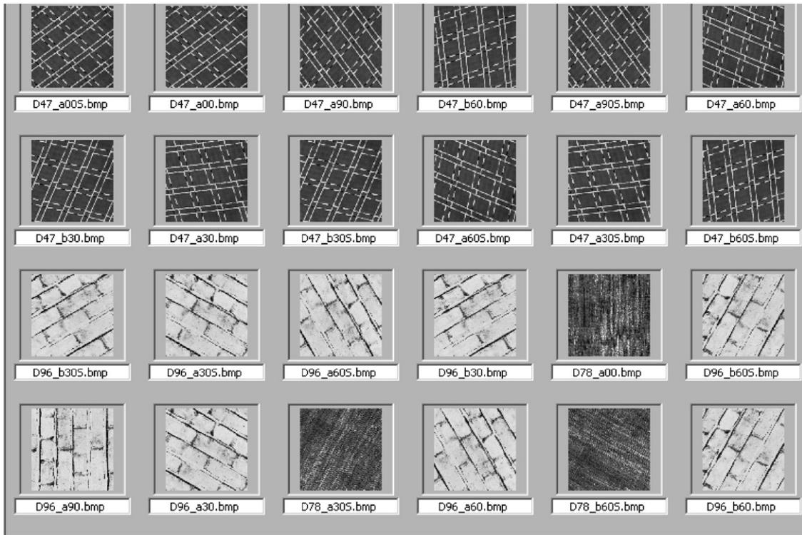
Fig. 2. An example for texture image retrieval based on SOH, which are displayed in a browser window. The test image is on the upper-left position and the retrieved images are listed in raster-scan order by descending similarity. The first 11 retrieved images are of the same subject with the test texture.
