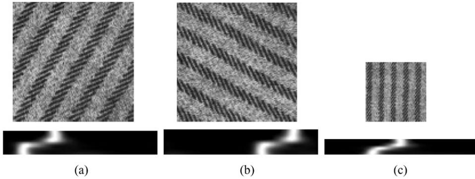
Fig. 1. The SOHs of three texture images: (a) original D11 texture, (b) rotated D11, and (c) zoomed D11. The texture images are listed in the first row and below them are their corresponding histograms, in which the vertical and horizontal axes represent the scale factor and orientation angle, respectively.
