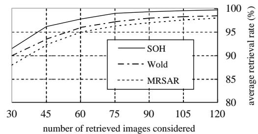
Fig. 3. The average retrieval rates between our algorithm, Wold decomposition and MRSAR over the database by considering from 30 to 120 top retrieved images.
