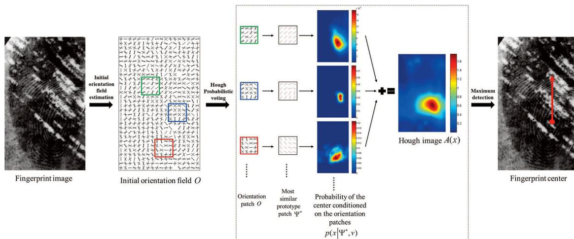
Fig. 10. Flowchart of estimating the finger center of an upright latent fingerprint.
