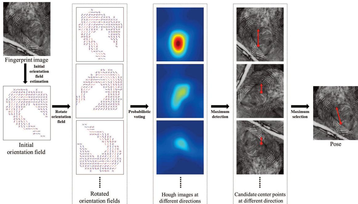
Fig. 11. Pose estimation of a fingerprint with unknown direction. The initial orientation field is rotated by a set of possible angles; the center estimation procedure is then applied to detect the center at each angle; and finally the one with the largest value is chosen.
