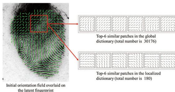
Fig. 14. Different lookup results of global dictionary and localized dictionary for a noisy initial orientation patch (marked by the red box). Because the initial orientation patch is very noisy, none of the top six similar patches in the global dictionary is close the true ridge orientations. But the top six similar patches in the localized dictionary contain several good estimates.
