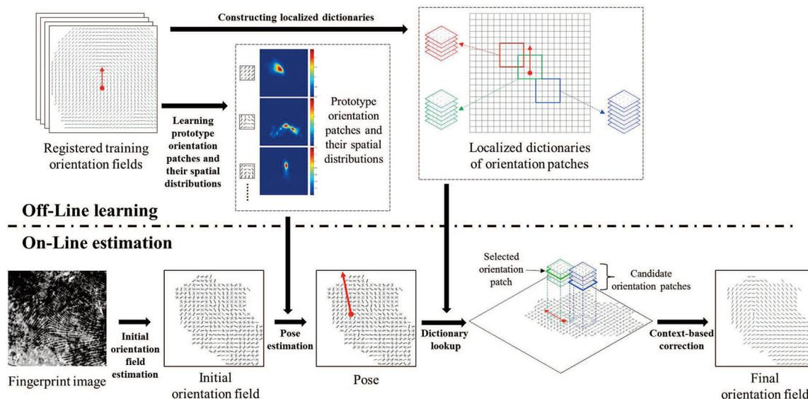
Fig. 3. Flowchart of the proposed fingerprint pose estimation and orientation field estimation approach. The approach is composed of two relatively independent parts. The first part is the off-line learning algorithm, while the second part is the on-line estimation algorithm.
