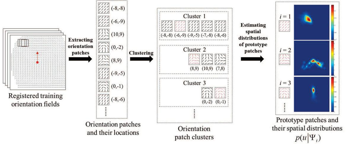
Fig. 8. Flowchart of learning a set of prototype orientation patches and their spatial distributions.
