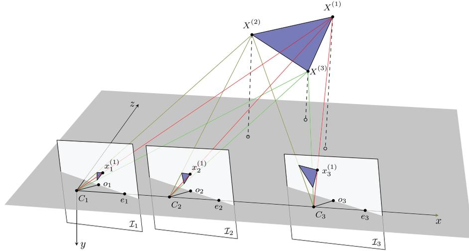
Fig. 2. 3D geometry of the sliding camera system. It can also be treated as many cameras on a track which are parallel and co-linear.
