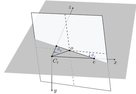
Fig. 4. Geometry relationship between  $e$  and  $\mathbf{R}$ .
