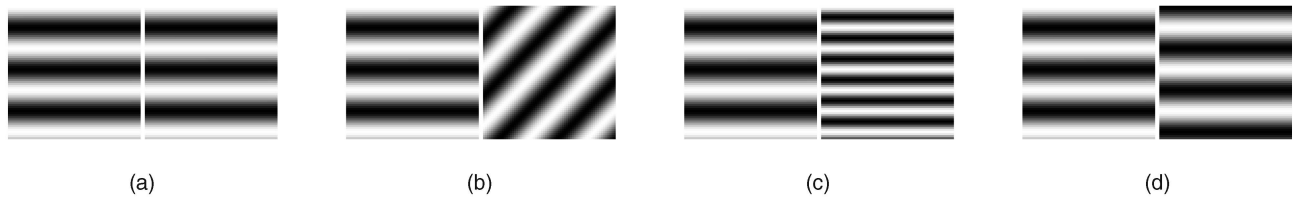
Fig. 6. Continuity of adjacent waves. (a) Two waves are continuous, (b) the direction of two waves is discontinuous, (c) the frequency of two waves is discontinuous, and (d) the normalized gray-scale values of two waves are discontinuous.
