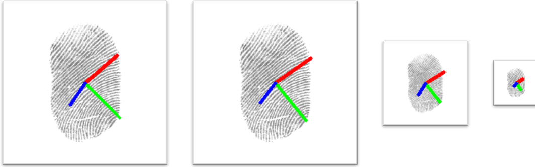
Fig. 10. Fingerprints of different resolutions. From left to right, they are 218 ppi image with ground truth, 218 ppi image with prediction, 109 ppi image with prediction, and 55 ppi image with prediction. The axes in the rightmost image were blurry due to the low resolution.
