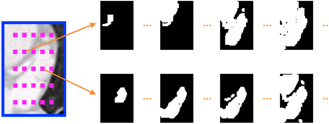
Fig. 6. Seed hypothesis. Small magenta squares represent different foreground seeds placed in rectangular grid. Blue lines on image borders represent background seeds. We also propose a segmentation scheme for two different foreground seed assumptions. In each cluster, \lambda increases from left to right with the image nodes tend to foreground. (For interpretation of the references to color in this figure legend, the reader is referred to the Web version of this article.)
