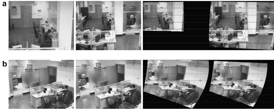
Fig. 10. Two spherical rectification experimental results. The left two images are the original images captured from the two PTZ cameras. The right two are the rectified images, whose sizes are normalized to that of the original image. The PTZ parameters: (a) PTZ_1 = [96.59 \ -12.45 \ 5.27] , PTZ_2 = [93.96 \ -18.08 \ 1.34] and (b) PTZ_1 = [127.48 \ -16.80 \ 2.35] , PTZ_2 = [123.58 \ -16.80 \ 2.35] .
