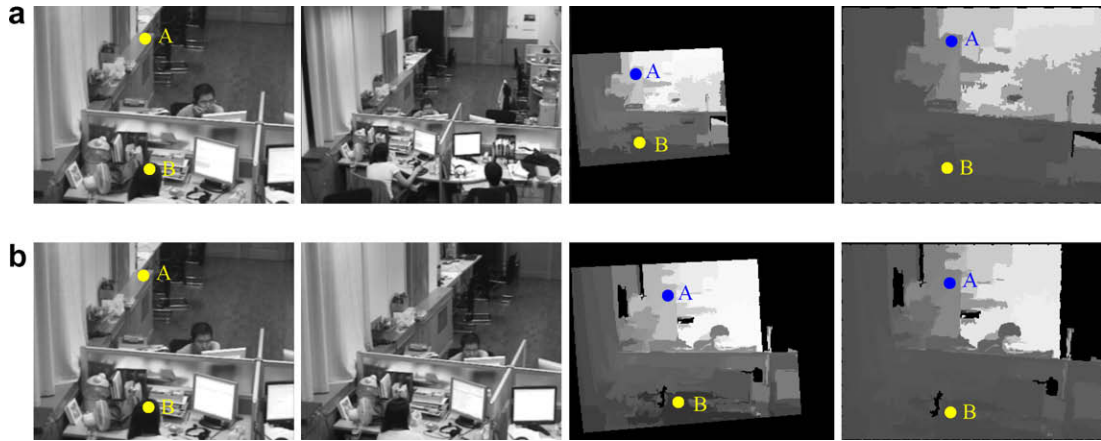
Fig. 12. Two experiments: depth map estimation of the same scene with different image pairs. The reference images of two experiments are identical, but the compared image of (a) has a lower zoom level than that of (b) (The specific parameters are in Table 3). A and B in images are testing points.
