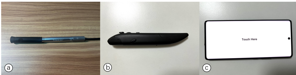
Fig. 10. The input devices used in the user study: (a) PalmPen; (b) a pen-shaped mouse; (c) a phone-based touchpad.
