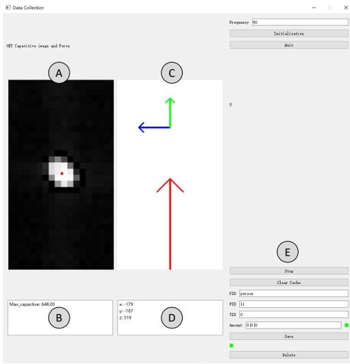
**Figure 3: The data collection program consisting of the normalized capacitive image (A) with the maximum capacitive value (B), visualization of the 3D forces (C) with raw force values (D), and the control buttons (E).**
